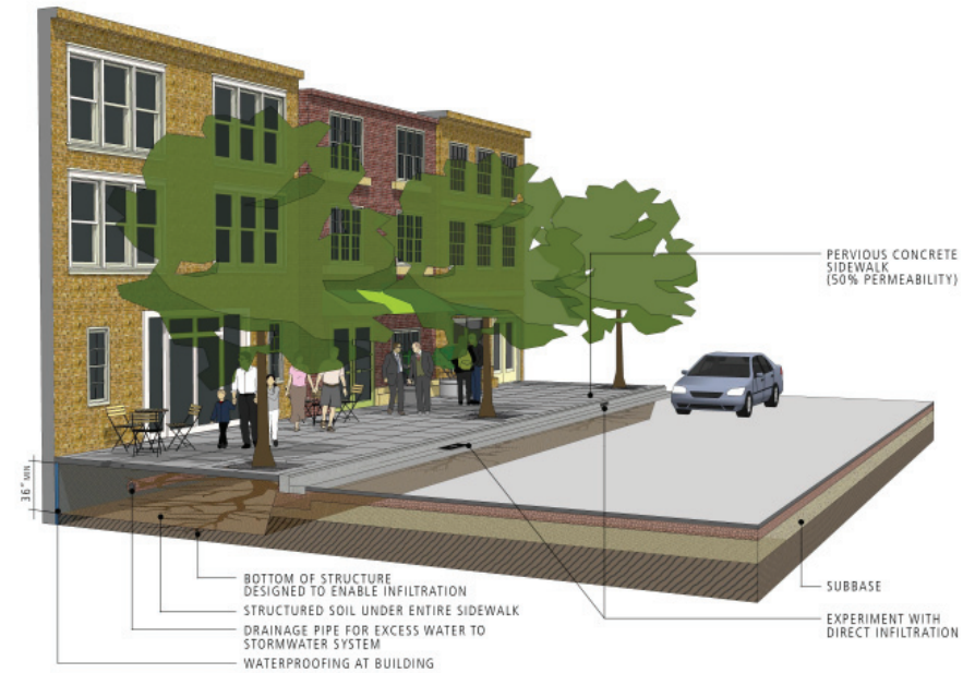
Figure 6.24- Example Streetscape Infiltration System
